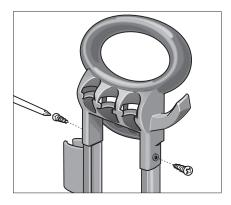
**Step 4** Insert each of the two short screws and tighten.
